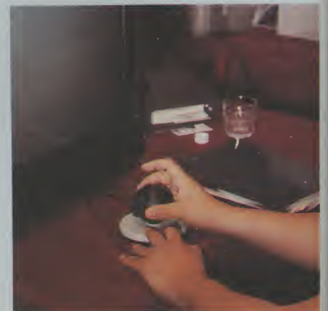
Using a GeoBall to control a screen display of a virtual world. The ball responds to pressure upwards and downwards, left and right, forward and backward, clockwise and anti-clockwise, giving 8D control – essential for manoeuvres in 3D space
